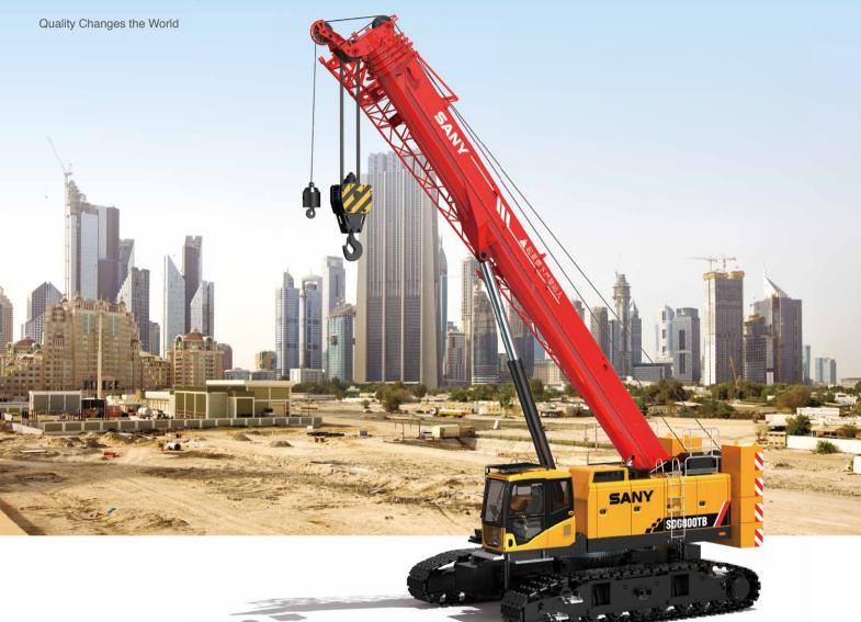
Max. lifting moment: 300t·m Max. boom length: 47m Max. boom + jib length: 47m+17.5m
